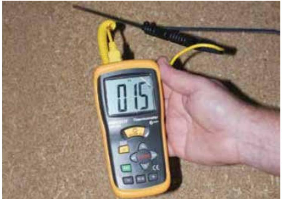
**Photo 4:** Use a digital probe to monitor moisture and temperature from both the top and the bottom of silos, if safe to do so.
