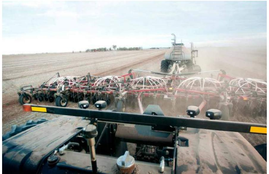
**Photo 4:** A New Holland T9 tractor with a Case Flexicoil PTX 600 airseeder bar towing a Flexi-Coil 3850 air cart bin used to sow cereal seed.
